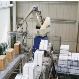
Palletizing robot handles max. 700 cases per hour. Direction of cases can be turn around, depending on characteristic of each product.
