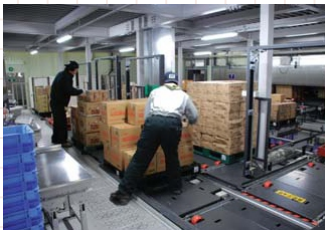
In the picking area, operators pick the quantity displayed on the terminal and induct onto the conveyor.
