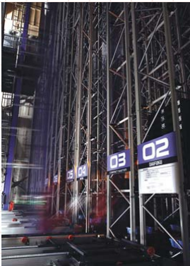
Six-crane unit load AS/RS stores 4,106 pallets (11,374 tons).
