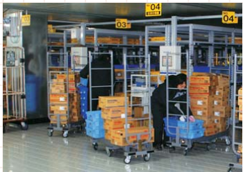
A piece sorting system sorts products by store. A single operator can sort 400 ~ 600 pieces/hour.
