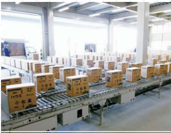
Receiving area with 7 in-line conveyors, put lids onto cases and ties them down automatically.
