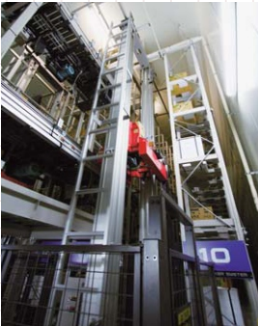
Mini load AS/RS (5 cranes, stores 1,090 cases). Upper conveyor delivers products to the AS/RS, and lower conveyor delivers products from AS/RS.
