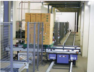
Shuttle STV. Transports pallets between palletizing robot, vacuum cooling storages, and unit load AS/RS.
