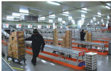
Case products sorted per route/store by the Jet Surfing Sorter and are transported on designated carts to the shipping accumulation area.
