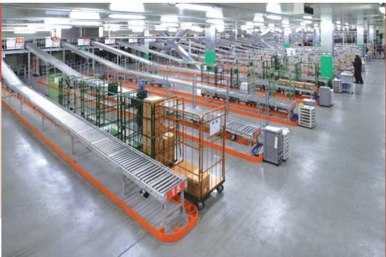
Sixteen-chute Jet Surfing Sorter sorts 4,000 cases/hour.
